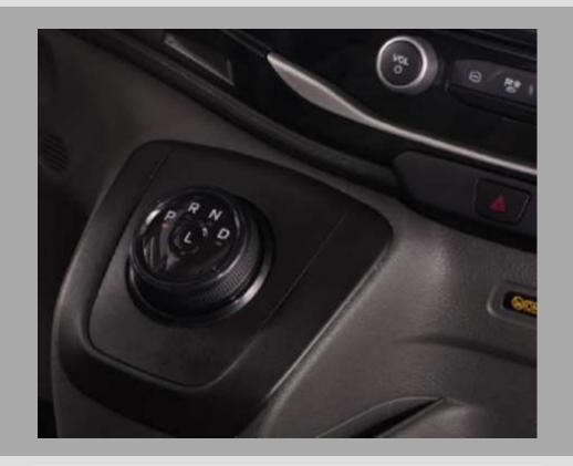
✓ Automatic transmission mounted on the console and steering wheel levers for manual selection.
